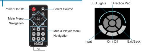
Both the keypad and remote can be used to navigate through the menus. The Main Menu Navigation on the remote functions exactly the same as the directional pad on the P300 unit.
