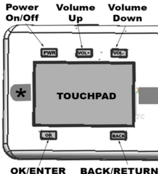
The P4X Android incorporates a capacitive touchpad directly onto the top of the projector. This touchpad works in conjunction with a pointer and allows users to select icons, APKs, and scroll through the menu system. Like most notebook touchpads, the touchpad can be double-tapped for a click or used in conjunction with the Enter and Back buttons below the touchpad.
