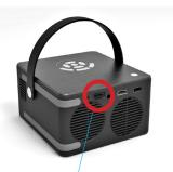
The P6U can read files directly from both a TF Card and USB Drive.
